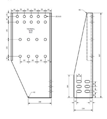
Use these side plates to install the coupling at the same height of the frame beam lower surface.
