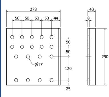
Use these side plates to install the coupling head at the height of the frame beam lower surface. Install the side plate with the strengthener bent forward. Delivered in pairs.
