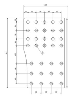
Install the coupling about 100 mm below the lower surface of the vehicle's frame with these side plates.
