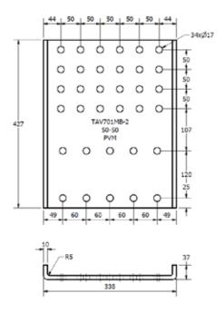
Install the coupling about 100 mm below the lower surface of the vehicles' frame with these side plates.
