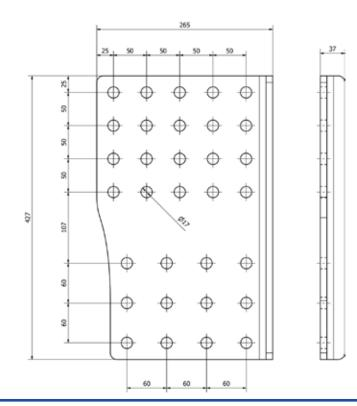
Install the coupling about 100 mm below the lower surface of the vehicle's frame with these side plates.
