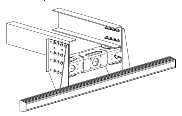
Install the underrun protection on the TAV702 side plates or, with separate fasteners, on the vehicle's frame.
