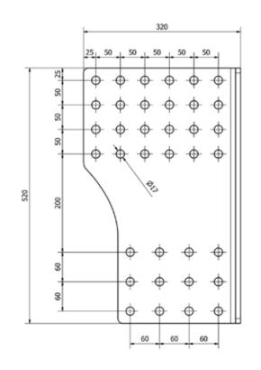
Install the coupling head about 200 mm below the frame with these side plates.
