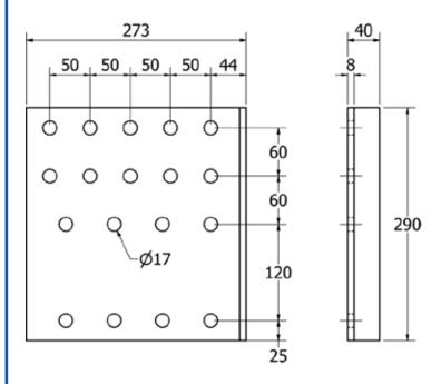
Use these side plates to install the coupling head at the height of the frame beam lower surface. Install the side plate with the strengthener bent forward. Delivered in pairs.
