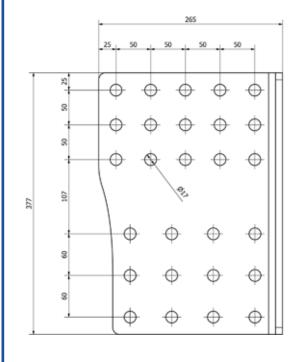
Install the coupling about 100 mm below the lower surface of the vehicle's frame with these side plates.
